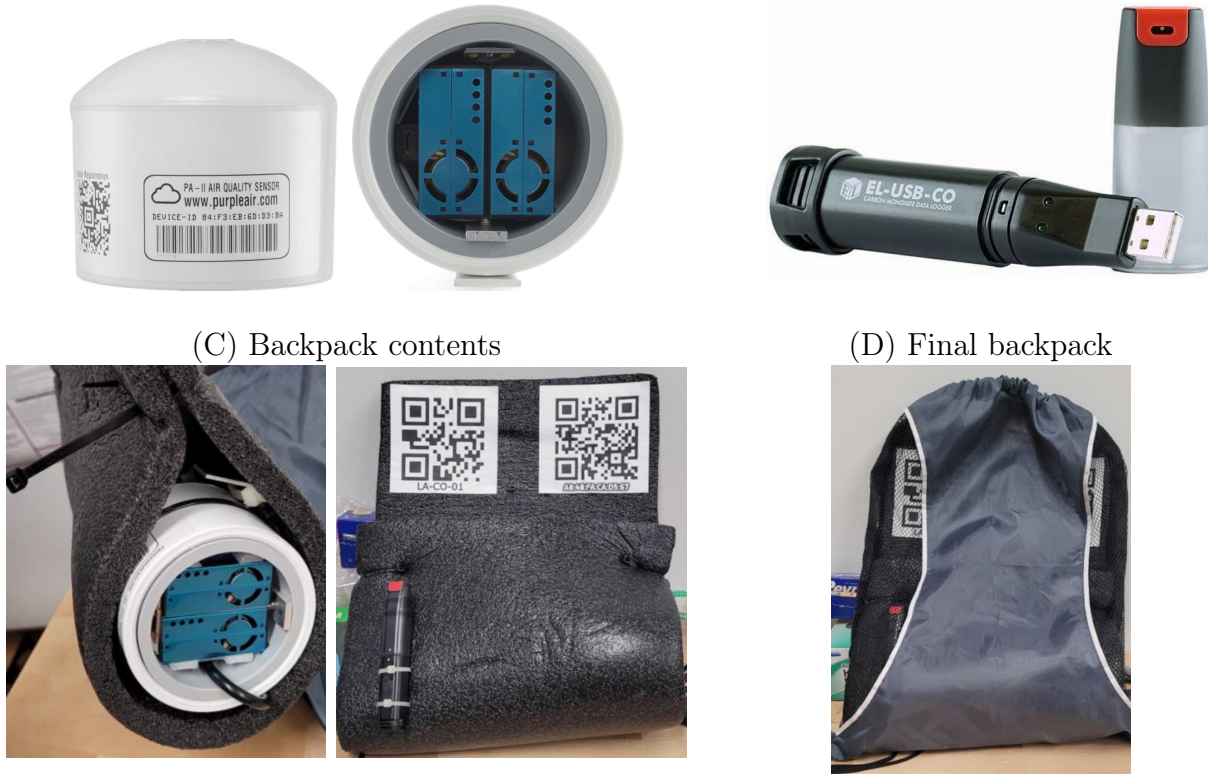
Figure A5: Devices to record air pollution and mesh backpacks containing them (A) Particulate Matter (B) Carbon Monoxide
